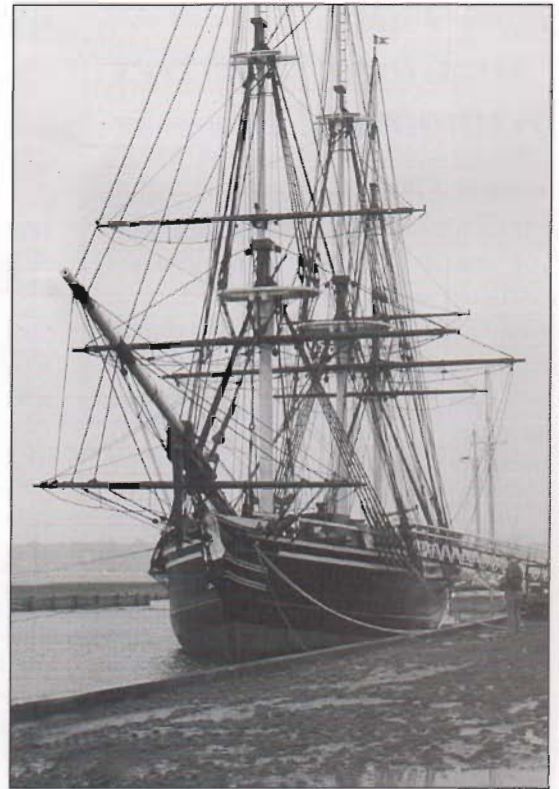
The "Friendship" is a reconstruction of a 171-foot, three-masted Salem East Indiaman built in 1797. She is the largest Coast Guard certified, wooden sailing vessel to be built in New England in more than a century.
